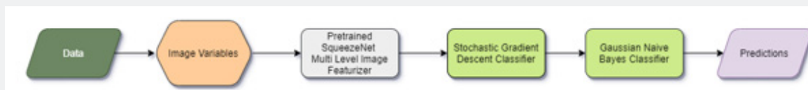
Figure 5: Stochastic Gradient Descent rice plant disease predictions become model inputs for Gaussian Naive Bayes Classifier.
